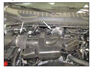
4. Loosen the hose clamps that secure the intake plenum to the air filter housing and to the throttle body, then remove the intake plenum from the vehicle.
