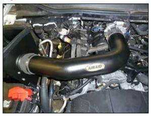
19. Install the AIRAID intake tube into the hump coupler and then into the step coupler at the throttle body, adjust the tube for best fit and then secure with the provided hose clamps.
