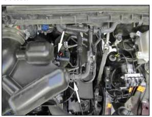
2. Release the spring clamp that secures the EVAP vent line to the intake plenum. Then release the locking tap on the Crankcase vent fitting and disconnect the crank case vent from the intake plenum.
