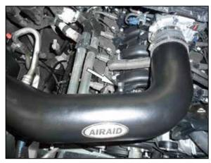
22. Install the longer vent hose assembly onto the AIRAID intake tube and then into the factory vent line as shown.
